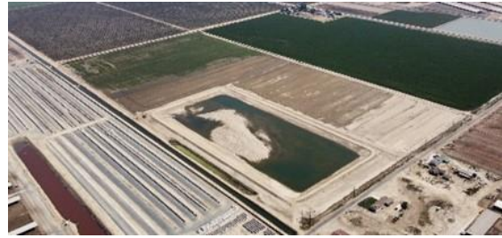
Figure 4 Establishing the MAR infiltration basin.
