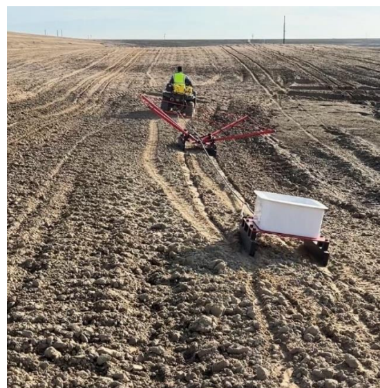
Figure 1. tTEM survey in central valley 2024 performed by GIP.
